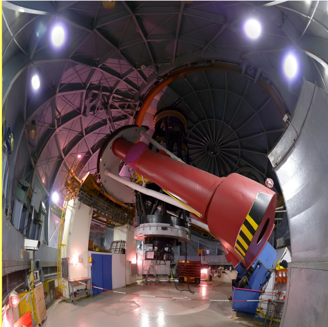
Fig. 9.21. View of the interior of the Bernard Lyot Telescope dome. The red structure is the horseshoe-shaped setting which supports the 2 m telescope. The NARVAL system can be seen, installed at the telescope's focus (2009). Photo © Paul Compère
